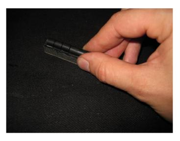
Slide the block of 12 pads off the rod. Place the canvas cloth on a flat surface and scrub the lambskin on the canvas. This will remove the thinner, looser fibers so that they won't shed off onto the reeds while in use. You will probably only need to rub for about 20-30 seconds.
