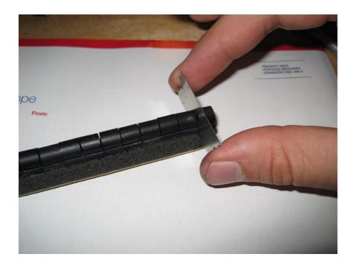
Using a razor blade, slice vertically through the dried weatherstrip adhesive and the foam rubber, being careful to keep the blade both vertical and square to the length of the block.
