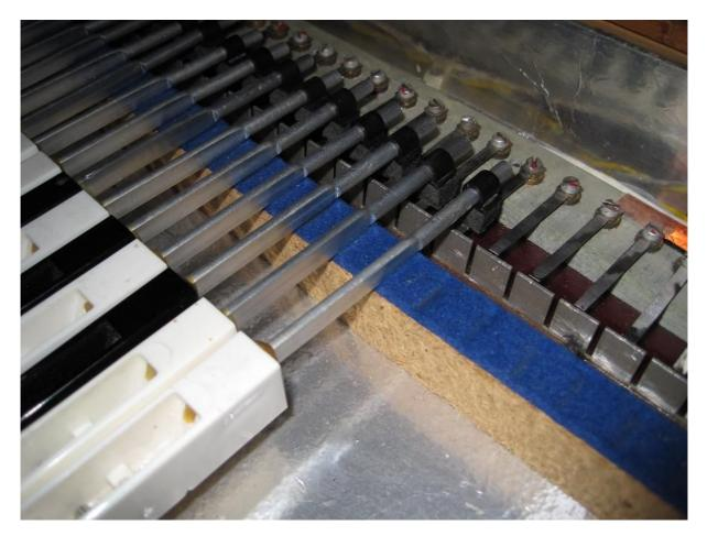
Slide the new pads onto the key shafts, lining them up with the marked locations of the old pads. If you don't have a record of where the original pads were placed, this photo shows them pretty clearly if you zoom in:
