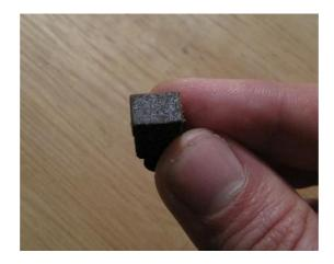
After the pads are done soaking, remove the excess grease by wiping them with a paper towel. You will want to wipe down the surface until it just barely starts to lose its gloss. I took a photo with no flash, holding the pad so that the lamp was reflecting on it, in order to show what it should look like.
