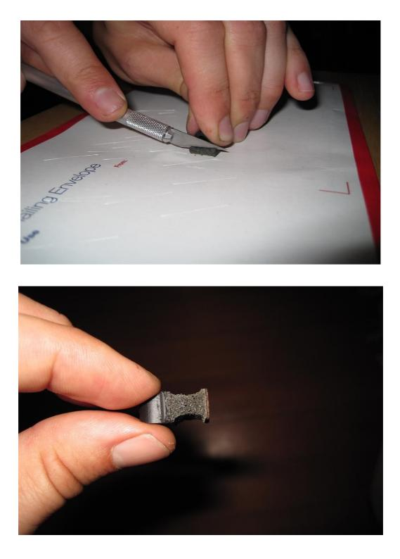
If you are starting from scratch with an untouched Pianet, you may find that these home-made pads are a bit too thick and stiff and require some of the key shafts, particularly on the black keys, to be bent up about 1/16" to 1/8". Alternatively, you can make the pads less stiff by following step 9.
